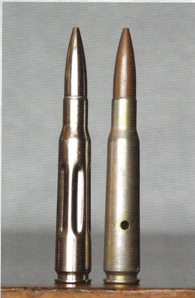
The new M2A1 Dummy round (left), plating by Advanced Plating Technologies, with the previous version, the M2 Dummy (right). The M2A1 is awaiting hole drilling in the case. Photo © 2014 by Keith Pagel
