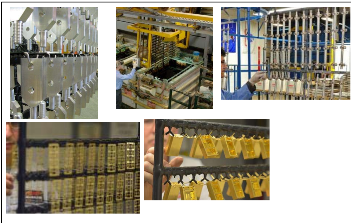
Figure 1.1 – Rack Plating Fixtures and Their Diversity
