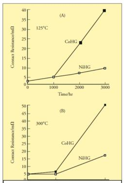
**Figure 1:** Contact resistance of Cobalt Hardened (CoHG) and Nickel Hardened (NiHG) gold deposits as a function of temperature and time.
