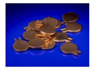
Nickel purity is critical as this layer is the functional bonding layer. For nickel soldering the higher purity nickel the better the soldering. Often plating companies use an organically brightened nickel layer such as a brightened Watts or sulfate-based nickel to give a bright finish at the expense of solderability. Advanced Plating Technologies offers an <a href="engineered sulfamate nickel-plating">engineered sulfamate nickel-plating</a> layer
